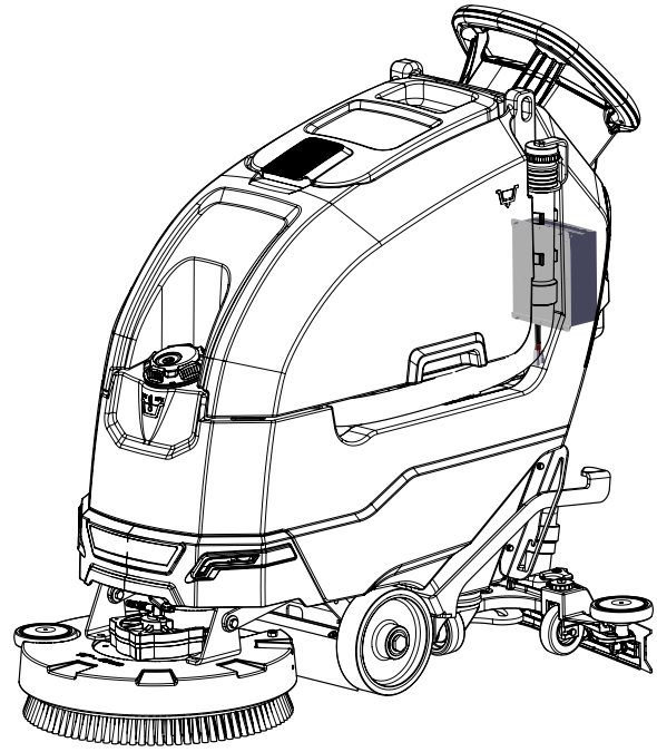
6 - ON-BOARD BATTERY CHARGER
